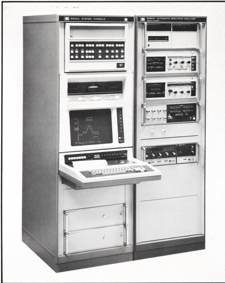
Fig. 1. Automatic Spectrum Analyzer (Model 8580A) can assume many configurations. This one is typical of those for use in automatic spectrum monitoring.
